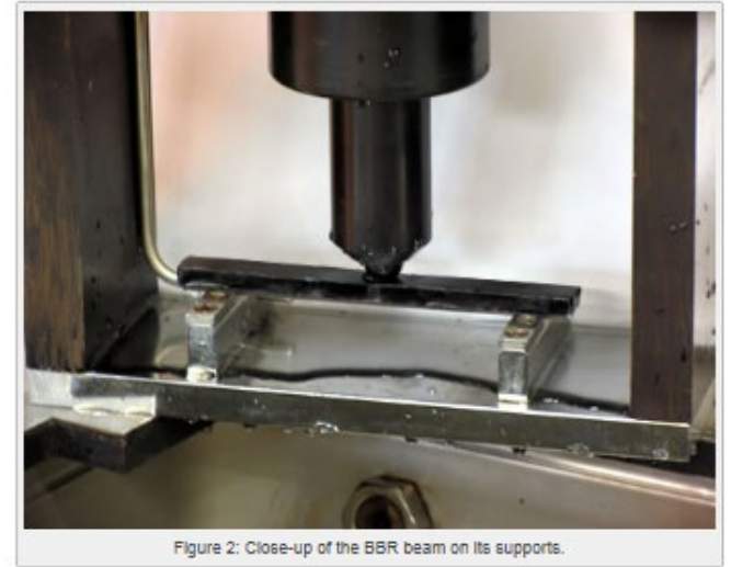
Figure 2: Close-up of the BBR beam on its supports.
