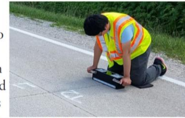
Figure 23. Ultrasonic pulse echo imaging of concrete overlays to analyze crack deployment
