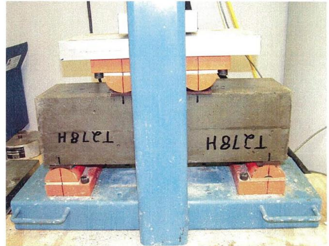
Figure 4 – Reaction Frame for Third-Point Flexural Beam Test (ASTM C78)
