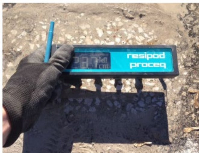
Figure 49. Surface resistivity testing on the bridge deck
