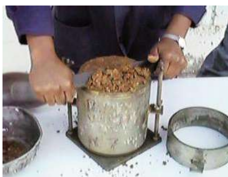
Figura 6.1_104. Enrase del Material
